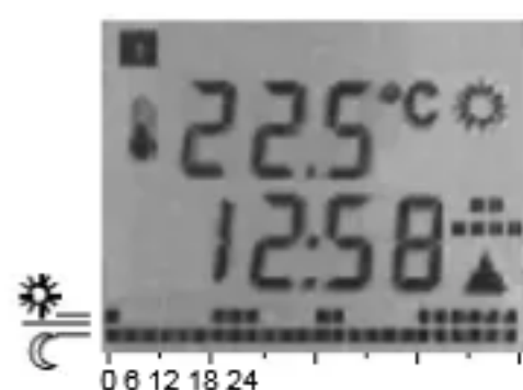
Automatic changeover according to the switching pattern
