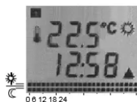
Automatic changeover according to the switching pattern
