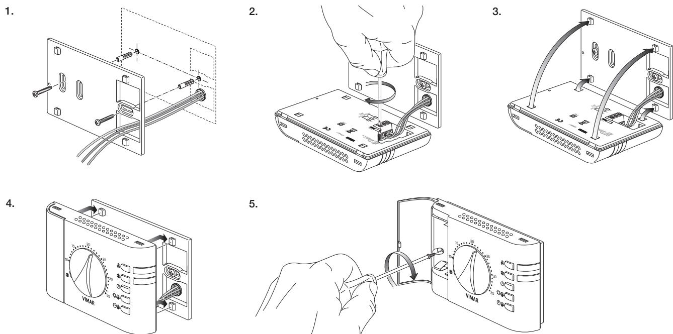
INSERIMENTO/SOSTITUZIONE BATTERIE • INSERTING/CHANGING THE BATTERIES • INSTALLATION/REEMPLACEMENT DES PILES
