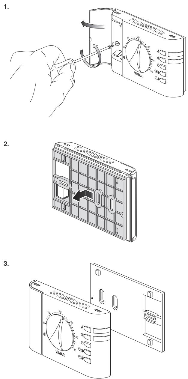
INSTALLAZIONE SOPRA SCATOLA DA INCASSO • MOUNTING ABOVE FLUSH-MOUNTING BOX • INSTALLATION SUR BOÎTE D'ENCASTREMENT
