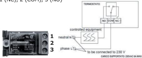
**IMPORTANT:** You can only and connect a single appliance (stove, fan, boiler). The connection of several equipment in cascade or in series (for example, a heater and a fan) does not guarantee the correct functioning of the device. Do not connect the thermostat to a conditioner/air conditioning.
